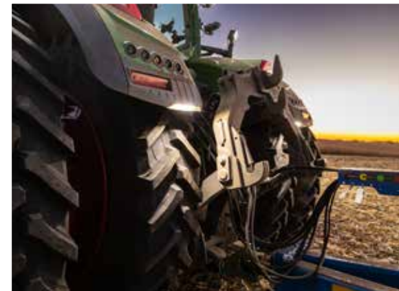
The 800 Vario Gen5 Series features new GroundVision drawbar lighting in the fenders, which perfectly illuminates the rear implement. This ensures you have the best visibility for attaching or unhooking implements and to monitor areas like a baler pick-up when working after dark.
