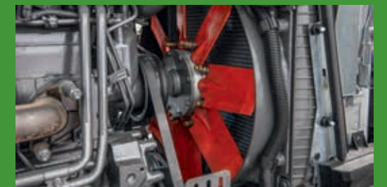
Reverse fan: for demanding conditions The optional reversing fan reduces daily maintenance tasks and increases machine uptime.
