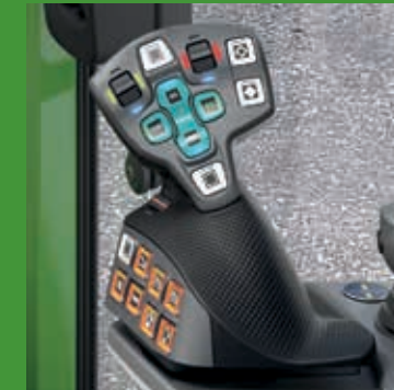
Driving pedal or joystick control: The driving mode can be selected individually. The speed can be controlled with either the pedal or the joystick. Change drive direction either with the joystick or the reverse lever with built-in stop and go function.
