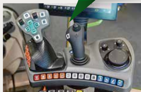
▲ The new driver's workstation with multifunction driving lever, 3L joystick and rotary push-button
