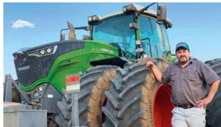
▲ Fanie in front of his Fendt 1050. The gaps between the front twin tyres are larger, so that stones don't get stuck between the tyres. On the farm we drive with very low air pressure in the tyres. Great for the soil!
