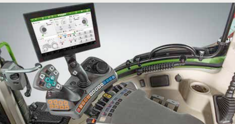
▲ The new driver's workstation with multifunction driving lever, 3L joystick and rotary push-button
