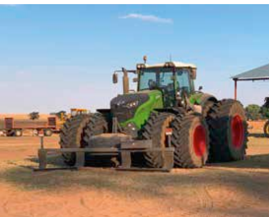
▲ The tractor drives mainly in the corn and the front attachment is designed to bend the corn stubble in the direction of travel, to spare the tyres.
