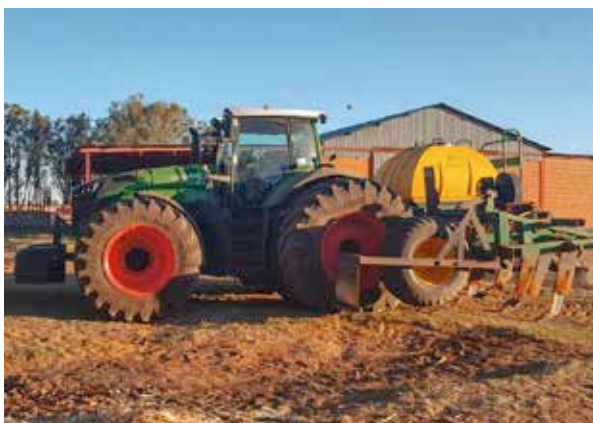
▲ The Fendt 1050 Vario has a 7-t subsoiler that works to depths of 80 cm. Mineral fertiliser is incorporated at the same time.
