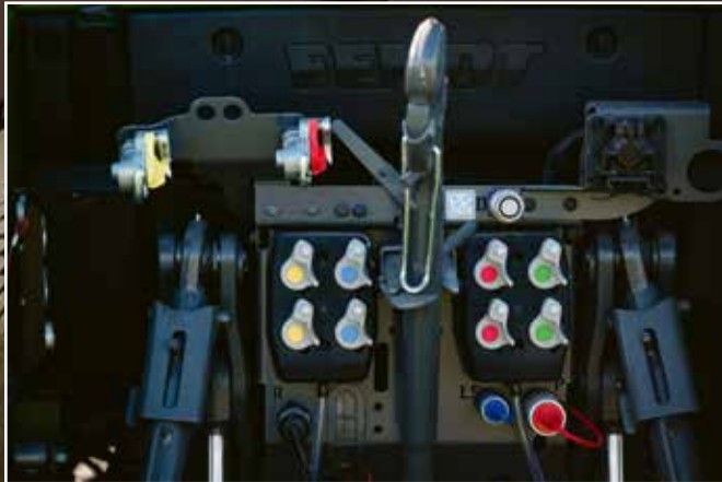
Self-closing dust caps protect connections on the front and rear of the tractor.
