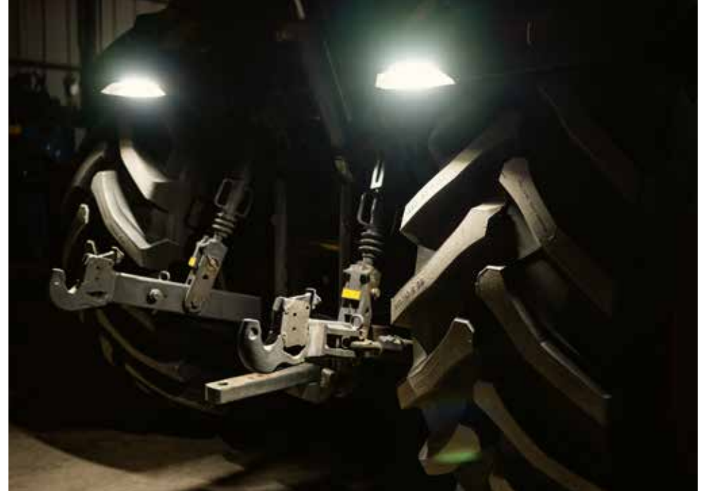
New GroundVision, included with all lighting packages, uses two LED lights in the rear fenders to light the hitch and front of the rear implement.
